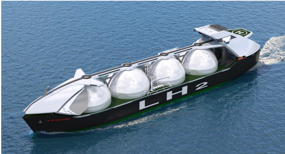
Figure 2: 160,000m 3 type LH2 carrier
